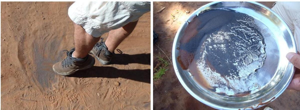
**Figure 4 – Left: Exposure of high grade mineral sands at Tajiri and Right: Simple panning of the sand results in easy separation of the black heavy mineral content.**
