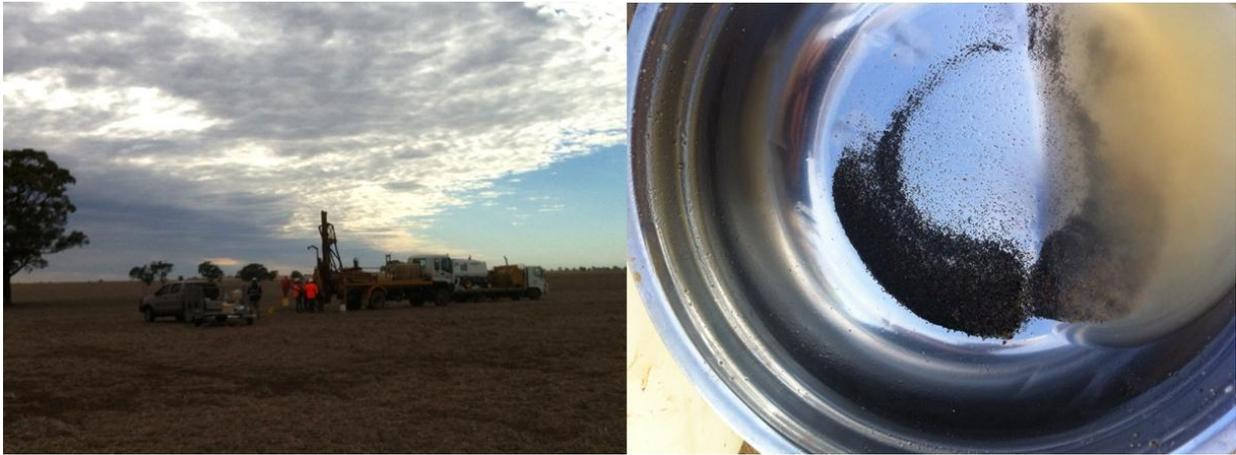
**Figure 2: Drill rig on site near Warracknabeal and a panned sample showing high grade HM**
